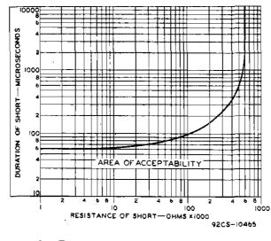
Fig.3 - Thyratron-Type Shorts Test for Type 7587.
