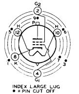
PIN 7: ▲ PIN 8: CATHODE PIN 9: ▲ PIN 10: HEATER PIN 11: OMITTED PIN 12: HEATER , CAP: PLATE
