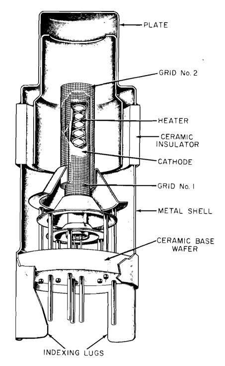
Fig.4 - Illustration of a nuvistor tetrode showing cylindrical electrodes and tripod-like supports.
