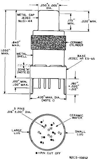
NOTE I: MAXIMUM O.D. OF 0.440" IS PERMITTED ALONG 0.190" LUG LENGTH. NOTE 2: SHELL TEMPERATURE SHOULD BE MEASURED IN ZONE "A" BETWEEN BROKEN LINES.
